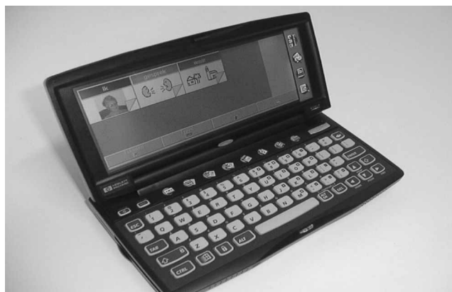
Figure 1. PCAD: portable communication aid for dysphasic people.
